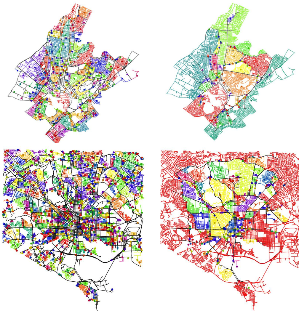
Figure 1: Automated generation of Superblocks. Athens (top row) and Baltimore (bottom row) Superblocks generated using the residential partitioner (left column) and the betweenness partitioner (right column). The streets of each Superblock are colored, the rest of the streets are black. Colored nodes denote representative nodes within each Superblock for easier visual recognition. Map data from OpenStreetMap.
